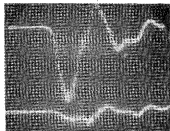
Fig. 10. Performance of the AND circuit when the two inputs are separated by about 600 ps. The output of the AND circuit along with the inputs to the two TELD gates and the output of one of the two TELD gates is shown here. The output of the AND circuit is “0” as the outputs of the two gates are not in coincidence. (a) Input. (b) Output.
